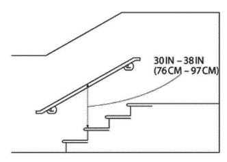
Figure D-12 - Handrail Measurement
